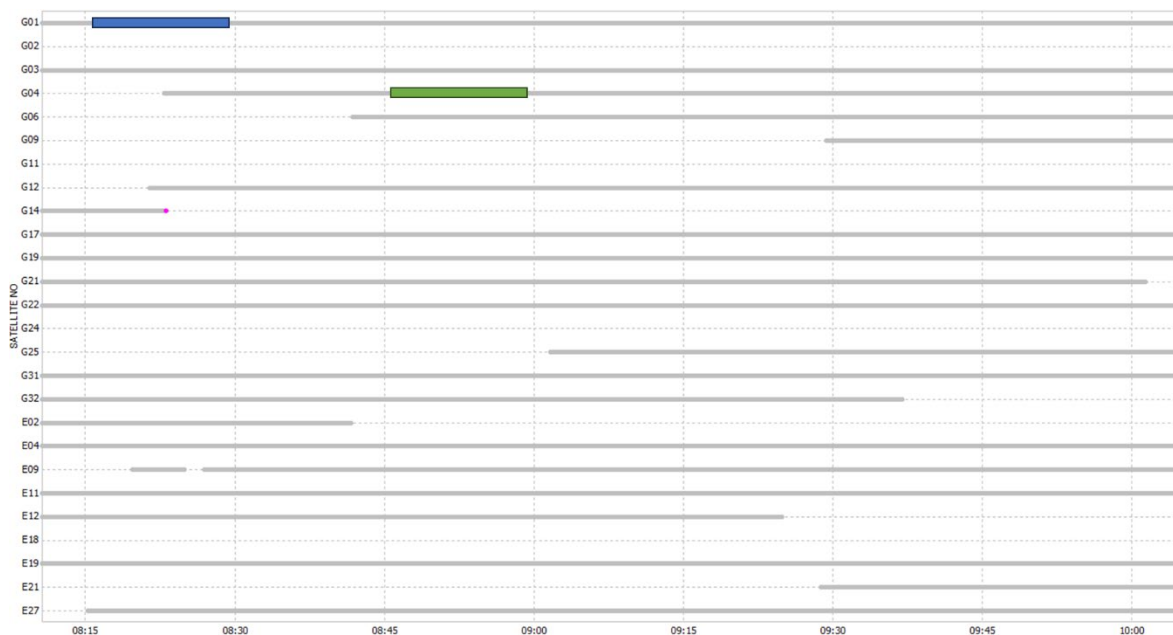
Figure 6-1 Satellite visibility condition and Fault injected on satellite G01 at time = 08:16:56 (844s) to 08:21:26 (1144s) and G04 at time = 08:45:30 (2558s) to t = 08:50:30 (2858s)
