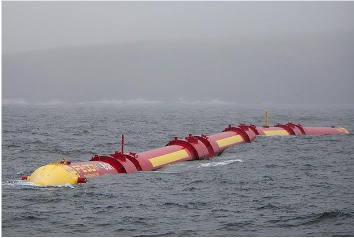
Figure 5 – Pelamis P2 device, pictured at European Marine Energy Centre, Orkney, in July 2011.
