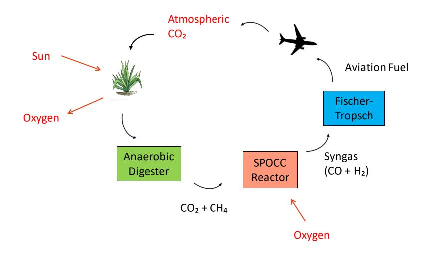
Processes which release CO<sub>2</sub>, and could benefit from the SPOCC Reactor:-
