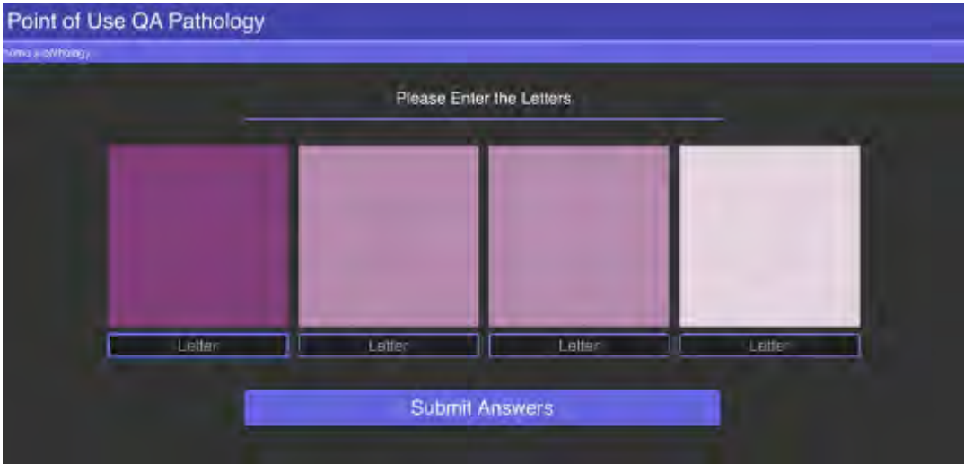
Figure 7: Point of Use QA is a simple point-of-use quality assurance tool for ensuring your display device allows you to see the minimum amount of visual contrast between colours, for scoring digital pathology slides. Data collected from this suggests an approximate 8% failure rate. The colours tested represent the most common pathological stain, H&E; pinks and purples
