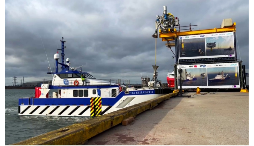
MJR Controls successfully completing harbour trials of their automated electric offshore vessel charging system following CMDC1 project.
